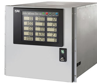
CPI 2500 W X-band TWT, Model T25XI-B
